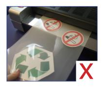
Never laminate small, cut-up pieces without using a Lifejacket® or you risk jamming and damaging your laminator (this will not be covered under warranty)
